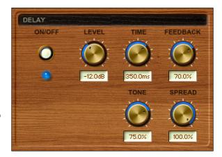
*Tone*: sets the high-frequency damping of the repetitions generated by the delay, where 0% provides no damping, and 100% provides full damping for a darker sound.
